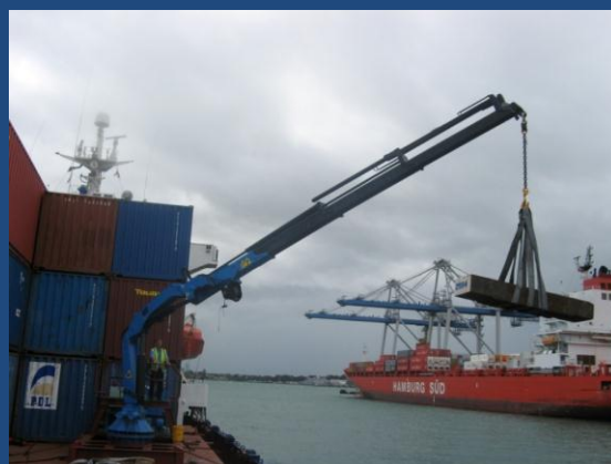
2184 kg test load lift at full 9.5 m extension
