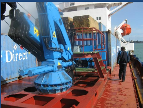
Crane mounted flat rack locked in position ready for load test
