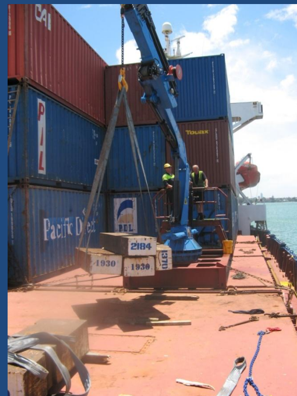
7414 kg certified test load lift
