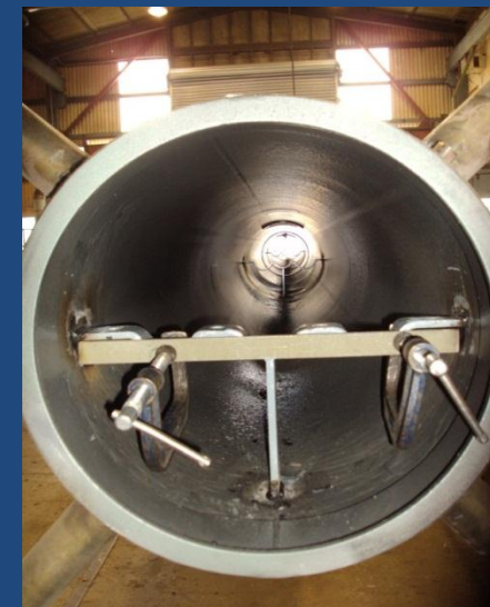
Mast being fabricated and Exhaust Brackets
