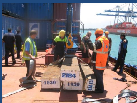
7414 kg certified test load ready for lifting
